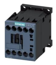
power contactor, AC-3e/AC-3, 7 A, 3 kW / 400 V, 3-pole, 110 V AC, 50 Hz / 120 V, 60 Hz, auxiliary contacts: 1 NC, screw terminal, size: S00, reusable packaging, pack = 144 units
