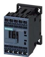
power contactor, AC-3e/AC-3, 7 A, 3 kW / 400 V, 3-pole, 24 V DC, 0.7-1.25\* Us, with integrated diode, auxiliary contacts: 1 NO, spring-loaded terminal, size: S00, suitable for PLC outputs, not expandable with auxiliary switch , reusable packaging, pack = 120 units
