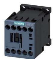
power contactor, AC-3e/AC-3, 12 A, 5.5 kW / 400 V, 3-pole, 110 V AC, 50 Hz / 120 V, 60 Hz, auxiliary contacts: 1 NO, screw terminal, size: S00, multi-unit packaging, pack = 72 units
