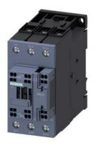
power contactor, AC-3e/AC-3, 51 A, 22 kW / 400 V, 3-pole, 24 V AC, 50 Hz, auxiliary contacts: 1 NO + 1 NC, main circuit: screw terminal, control and auxiliary circuit: spring-loaded terminal, size: S2, multi-unit packaging, pack = 15 units
