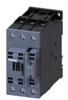
power contactor, AC-3e/AC-3, 51 A, 22 kW / 400 V, 3-pole, 24 V AC, 50 Hz, auxiliary contacts: 1 NO + 1 NC, main circuit: screw terminal, control and auxiliary circuit: spring-loaded terminal, size: S2, reusable packaging, pack = 30 units
