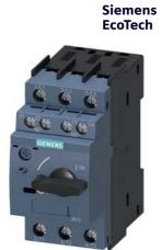
Circuit breaker size S00 for motor protection, CLASS 10 A-release 0.14...0.2 A N-release 2.6 A screw terminal Standard switching capacity with transverse auxiliary switches 1 NO+1 NC Reusable packaging Pack = 43 units
