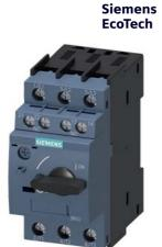
Circuit breaker size S0 for motor protection, CLASS 10 A-release 34...40 A Nrelease 480 A screw terminal Standard switching capacity with transverse auxiliary switches 1 NO+1 NC Reusable packaging Pack = 43 units
