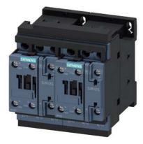
reversing contactor assembly, AC-3e/AC-3, 25 A, 11 kW / 400 V, 3-pole, 230 V AC, 50/60 Hz, screw terminal, electrical and mechanical interlock, auxiliary contacts: 2 x 1 NO, reusable packaging, pack = 20 units
