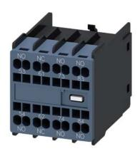
auxiliary switch, on the front, 3 NO + 1 NC, 53/54, 61/62, 73/74, 83/84, current path: 1 NO, 1 NC, 1 NO, 1 NO, spring-loaded terminal, for contactors 3RT2 and contactor relays 3RH2, reusable packaging, pack = 321 units
