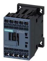
power contactor, AC-3e/AC-3, 12 A, 5.5 kW / 400 V, 3-pole, 24 V AC, 50/60 Hz, auxiliary contacts: 1 NO, spring-loaded terminal, size: S00, upright mounting position, reusable packaging, pack = 120 units
