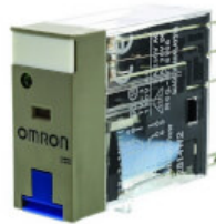
G2R-2-SNDI 48VDC (S) Relay, plug-in, 8-pin, DPDT, 5 A, mech & LED indicators, coil suppressor, lockable test button, label facility
