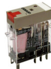
G2R-2-SNI 48VAC (S) Relay, plug-in, 8-pin, DPDT, 5 A, mech & LED indicators, lockable test button, label facility
