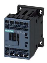
contactor relay railway 4 NO, 24-34 V DC, 0.7-1.25\*Us, with integrated varistor, spring-loaded terminal, frame size S00  $\,$
