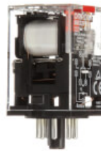
MKS2PIN 24VAC Relay, plug-in, 8-pin, DPDT, 10 A, mech & LED indicator, test button
