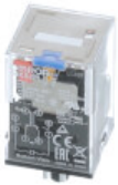
MKS2PIN 12VDC Relay, plug-in, 8-pin, DPDT, 10 A, mech & LED indicator, test button
