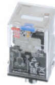
MKS2PIN 24VDC Relay, plug-in, 8-pin, DPDT, 10 A, mech & LED indicators, latchable test button, 24 VDC
