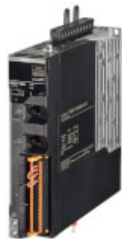
R88D-1SN02H-ECT-51 1S-51 servo drive with STO, SS1 and SLS safety, EtherCAT type, 200 W, 1 or 3~ 230 VAC
