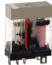
G2R-1-S 24VAC (S) Relay, plug-in, 5-pin, SPDT, 10 A, mech indicator, label facility, 24 VAC
