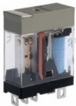
G2R-1-S 12VDC (S) Relay, plug-in, SPDT, 10 A, mechanical indicator, 12 VDC
