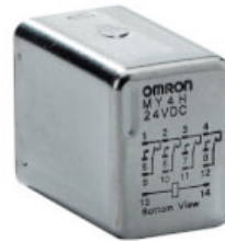
MY4ZH 24VDC Hermetically-sealed relay, plug-in, 14-pin, 4PDT, 3 A, bifurcated contacts
