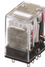
MY4ZN 110/120VAC (S) Relay, plug-in, 14-pin, 4PDT, bifurcated contacts, 5 A, mech & LED indicators, label facility, 110/120 VAC
