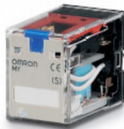
MY4ZIN 24VDC (S) Relay, plug-in, 4PDT (bifurcated), 3 A, mech. + LED indicator, test button, 24 VDC
