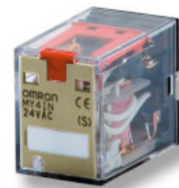
MY4Z 220/240VAC (S) Relay, plug-in, 14-pin, bifurcated contacts, 4PDT, 5 A, mech indicator, label facility, 220/240 VAC
