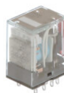
MY4ZIN-D2 24VDC (S) Relay, plug-in, 14-pin, 4PDT, bifurcated contacts, 5 A, mech & LED indicators, coil suppressor, lockable push to test button, label facility, 24 VDC
