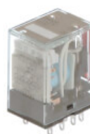
MY4ZIN-D2 24VDC (S) Relay, plug-in, 14-pin, 4PDT, bifurcated contacts, 5 A, mech & LED indicators, coil suppressor, lockable push to test button, label facility, 24 VDC
