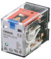
MY4IN-GS-R DC24 Relay, plug-in, 14-pin, 4PDT, 6 A, mechanical & LED indicators, lockable push test button, 24 VDC
