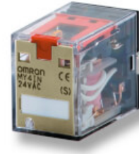
MY4ZIN 220/240VAC (S) Relay, plug-in, 4PDT (bifurcated), 3 A, mech. + LED indicator, test button, 220/240 VDC
