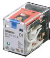
MY4IN-GS-R DC48 Relay, plug-in, 14-pin, 4PDT, 6 A, mechanical & LED indicators, lockable push test button, 48 VDC
