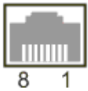
Fig. 9: Ethernet interface, pin numbering.
