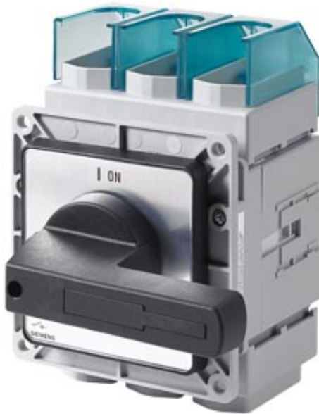
MAIN SWITCHES 3-POLE FRONT MOUNTING 4-HOLE MOUNTING CONTROL ELEMENT BLACK IU=250A P/AC-23A AT 400V=132KW
