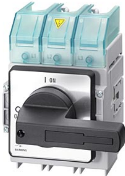
MAIN CONTROL SWITCH 3-POLE FLOOR MOUNTING KNOB OPERATING MECHANISM BLACK IU=250A P/AC- 23A AT 400V=132KW
