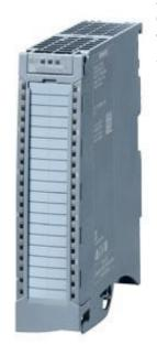
SIPLUS S7-1500 AI 8XU/R/RTD/TC HF 0 ... +60°C with conformal coating based on 6ES7531-7PF00-0AB0 . Analog Input Module AI 8 X U/R/RTD/TC HF, 16 BITS OF RESOLUTION, Accuracy 0.1%, 8 Channels in "groups of 1; common mode" Voltage: 30 V AC/60 V DC, "Diagnosis, Process alarms;" incl. infeed element, Shield clamp and Shield terminal
