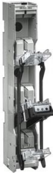
IN-LINE FUSE SWITCH DISCONNECTOR 3-POLE SWITCHABLE, SIZE 3, I=630A , U=690V, SCREW TERMINAL M 12 NEW DESIGN
