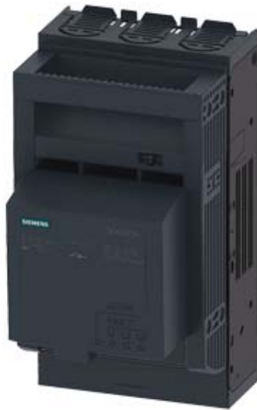
FUSE-SWITCH-DISCONNECTOR 3-POLE, NH00, 160A MOUNTING PLATE CONSTRUCTION COVER LEVEL 45 MM FLAT CONNECTOR FUSE MONITORING ELECTRONIC, EFM 10
