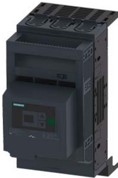
FUSE-SWITCH-DISCONNECTOR 3-POLE, NH00, 160A 40MM BUSBAR SYSTEM COVERS FOR RITTAL FLAT CONNECTOR FUSE MONITORING ELECTRONIC, EFM 20
