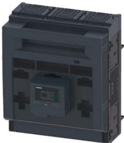
FUSE-SWITCH-DISCONNECTOR 3-POLE, NH3, 630A 60MM BUSBAR SYSTEM COVER LEVEL 32/70 MM FLAT CONNECTOR FUSE MONITORING ELECTRONIC, EFM 20
