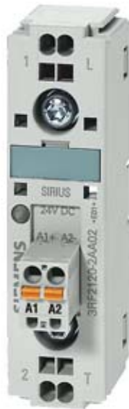
SEMICONDUCTOR RELAY 3RF2, 1-PH. WIDTH 22.5MM, 50 A 48-460 V / 110-230 V AC SPRING-LOADED TERMINAL
