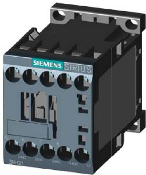
CONTACTOR RELAY, 3NO+1NC, AC 110V 50HZ, 120V 60HZ, SIZE S00, SCREW TERMINAL
