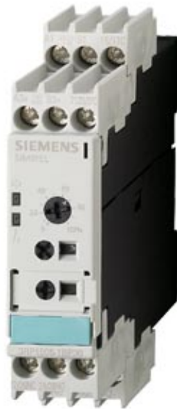
MULTI-FUNCTION TIME RELAY CAGE CLAMP TECHNIQUE 1 CHANGEOVER CONTACT WITH OFF- DELAY 0.5S...10S AC/DC 24V/AC 200...240V
