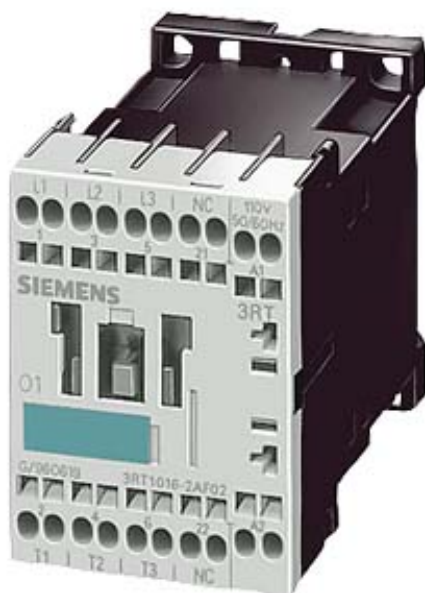
CONTACTOR, AC-3 5.5 KW/400 V, 1 NC, AC 24 V, 50/60 HZ, 3-POLE, SIZE S00, CAGE CLAMP CONNECTION
