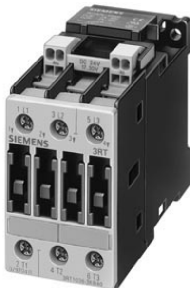
CONTACTOR, AC-3 11 KW/400 V, AC 24 V, 50 HZ, 3-POLE, SIZE S0, CAGE CLAMP
