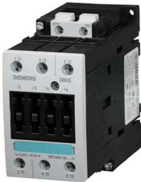
CONTACTOR, AC-3 15 KW/400 V, DC 220 V, 3-POLE, SIZE S2, SCREW CONNECTION
