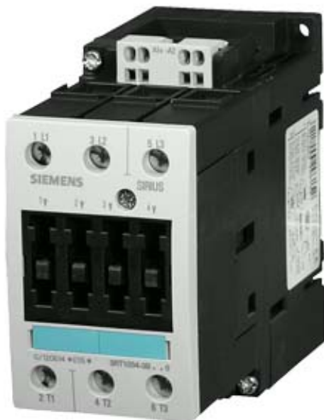
CONTACTOR, AC-3 15 KW/400 V, DC 24 V, 3-POLE, SIZE S2, CAGE CLAMP
