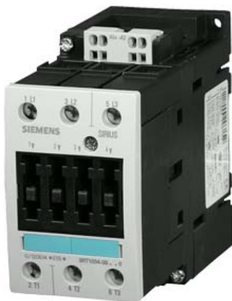
CONTACTOR, AC-3 18.5 KW/400 V, DC 48 V, 3-POLE, SIZE S2, CAGE CLAMP
