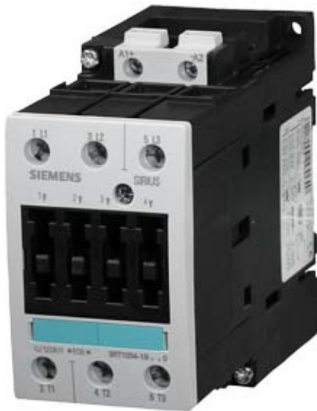
CONTACTOR, AC-3 22 KW/400 V, DC 42 V, 3-POLE, SIZE S2, SCREW CONNECTION
