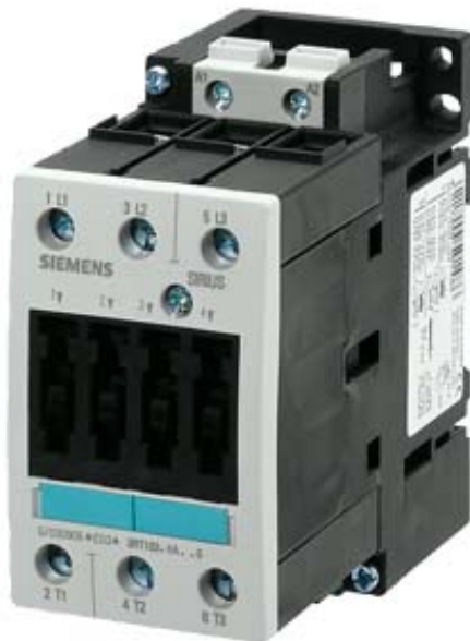
CONTACTOR, 3PH, 22 KW/400 V, 120 V AC, 60 HZ, 0.7...1.1 US 3-POLE, SIZE S2, SCREW TERMINAL
