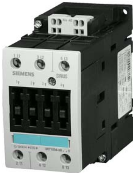
CONTACTOR, AC-3 22 KW/400 V, DC 42V, 3-POLE, SIZE S2, CAGE CLAMP
