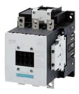
CONTACTOR, 90KW/400V/AC-3, AC(40...60HZ)/DC OPERATION UC 110...127V AUXIL. CONTACTS 2NO+2NC 3-POLE, SIZE S6 BAR CONNECTIONS CONVENTION. OPERATING MECHANISM SCREW TERMINAL
