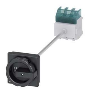
SENTRON, Switch disconnector 3LD, main switch, 3-pole, Iu: 63 A, Operating power / at AC-23 A at 400 V: 22 kW, floor mounting with door coupling, rotary operating mechanism, black, 4-hole mounting of the handle, without tolerance compensation
