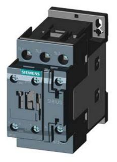
CONTACTOR, AC-3, 7.5KW/400V, 1NO+1NC, AC 230V 50/60HZ, 3-POLE, SZ S0 SCREW TERMINAL
