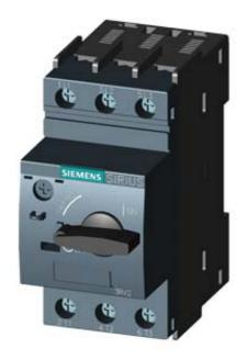
CIRCUIT-BREAKER SZ S00, FOR MOTOR PROTECTION, CLASS 10, A-REL.1.1...1.6A, N-RELEASE 21A, SCREW CONNECTION, STANDARD SW. CAPACITY
