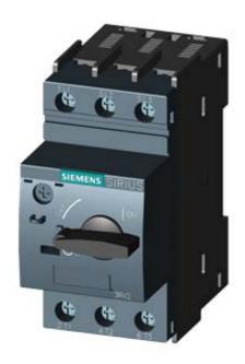
CIRCUIT-BREAKER SZ S00, FOR MOTOR PROTECTION, CLASS 10, A-RELEASE 4.5...6.3A, N-RELEASE 82A SCREW CONNECTION, STANDARD SW. CAPACITY
