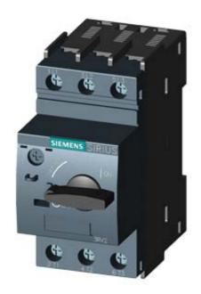
CIRCUIT-BREAKER SZ S00, FOR MOTOR PROTECTION, CLASS 10, A-RELEASE 5.5...8A, N-RELEASE 104A, SCREW CONNECTION, STANDARD SW. CAPACITY
