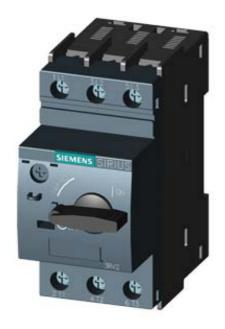
CIRCUIT-BREAKER SZ S0, FOR MOTOR PROTECTION, CLASS 10, A-REL. 3.5...5A, N-REL. 65A SCREW CONNECTION, STANDARD SW. CAPACITY
