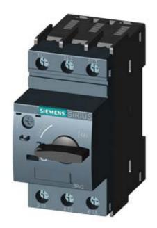
CIRCUIT-BREAKER SZ S0, FOR MOTOR PROTECTION, CLASS 10, A-REL. 5.5...8A, N-REL. 104A SCREW CONNECTION, STANDARD SW. CAPACITY
