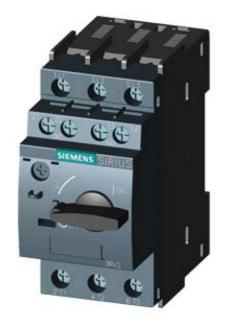
CIRCUIT-BREAKER SZ S0, FOR MOTOR PROTECTION, CLASS 10, A-RELEASE 11...16A, N-RELEASE 208A, SCREW CONNECTION, STANDARD SW. CAPACITY, W. TRANSVERSE AUX. SWITCH 1NO+1NC
