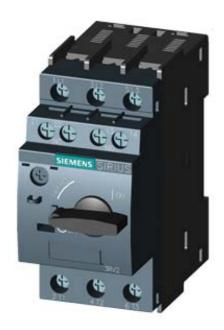
CIRCUIT-BREAKER SZ S0, FOR MOTOR PROTECTION, CLASS 10, A-RELEASE 17...22A, N-RELEASE 286A, SCREW CONNECTION, STANDARD SW. CAPACITY, W. TRANSVERSE AUX. SWITCH 1NO+1NC
