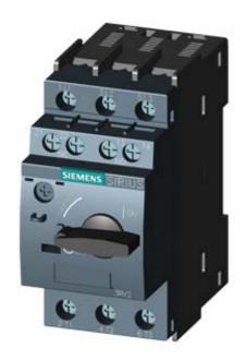
CIRCUIT-BREAKER SZ S0, FOR MOTOR PROTECTION, CLASS 10, A-RELEASE 20...25A, N-RELEASE 325A, SCREW CONNECTION, STANDARD SW. CAPACITY, W. TRANSVERSE AUX. SWITCH 1NO+1NC
