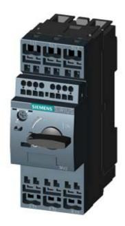
CIRCUIT-BREAKER SZ S0, FOR MOTOR PROTECTION, CLASS 10, A-RELEASE 23...28A, N-RELEASE 364A, SPRING-L. CONNECTION, STANDARD SW. CAPACITY, W. TRANSVERSE AUX. SWITCH 1NO+1NC
