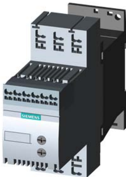
SIRIUS SOFT STARTER, SIZE S00, 12.5A, 5.5KW/400V, 40 DEGREES, 200-480V AC, 24V AC/DC, SPRING-LOADED TERMINALS
