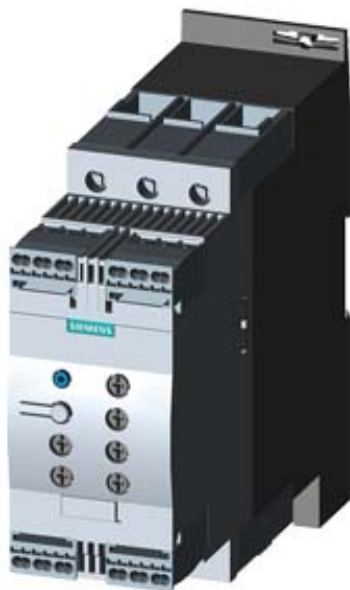
SIRIUS SOFT STARTER, S2, 63A, 37KW/500V, 40 DEGR., AC 400-600V, AC/DC 24V, SPRING-LOADED TERMINALS
